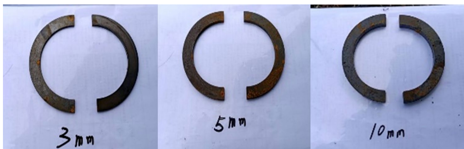
Fig. 18 Photos of split steel rings with different thicknesses that were used in this study
